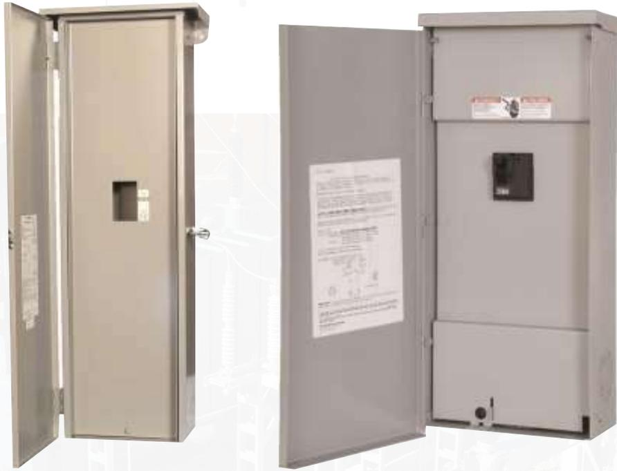
Enclosed circuit breaker is a reliable switching device which is used in residential, commercial, and industrial applications. It protects a circuit under overload or short circuit conditions depend upon the breakers used. Also characterized by the complete isolation of the circuits for safety when conducting Maintenance. Various sizes of knockouts are available on both sides for top and bottom entry of cables. It is available for indoor and outdoor application.
